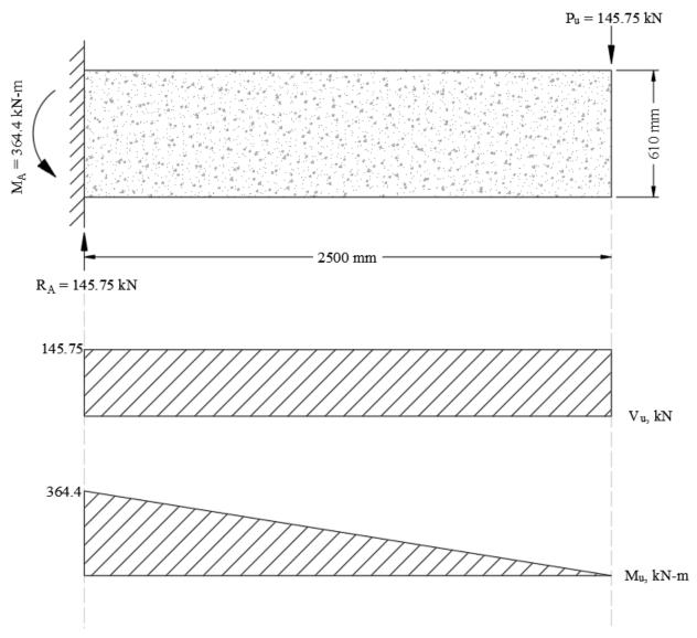
Figure 2 – Shear and Bending Moment Diagrams
