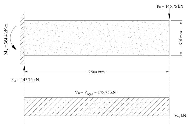
Figure 4 – Shear Diagram for Cantilever Beam
