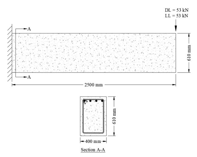
Figure 1 – Rectangular Reinforced Concrete Cantilever Beam
