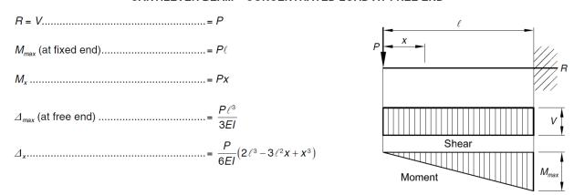
Figure 3 - Design Aid Tables (Beam Design Equations and Diagrams) - PCI Design Handbook
